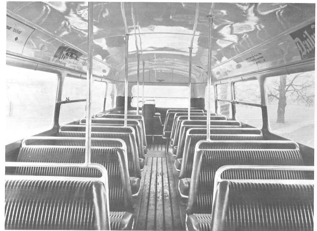
Top deck interior of RT bus, 1939. The almost seamless finish was one of the most successful examples of London Transport's pre-war design policy.
